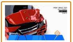
Engineers build cars with special crumple zones. The crumple zone absorbs the impact. This reduces the amount of energy transferred to passengers during a crash.
